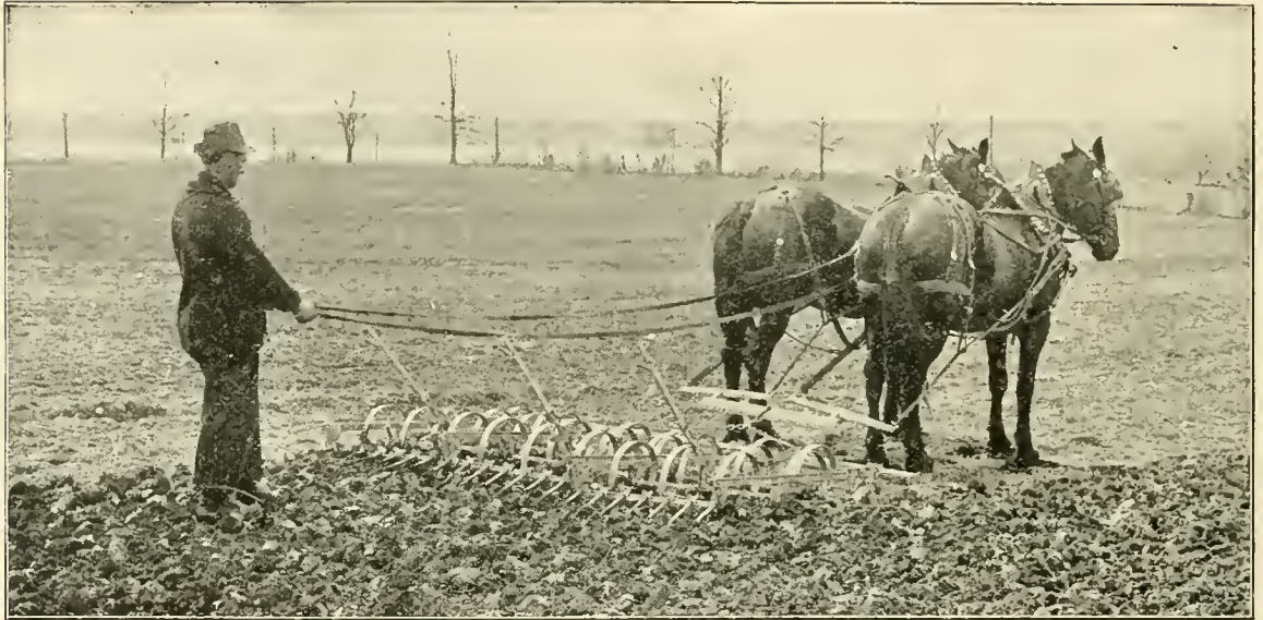
The McCormick combination harrow does the work of a spring-tooth and a peg-tooth harrow in one operation
