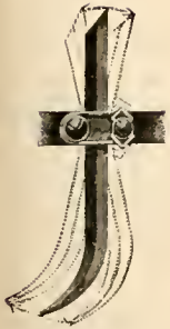
The teeth on the 14-tooth cultivator are adjustable
