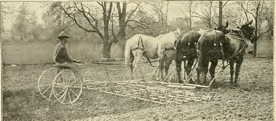
The riding attachment is connected to the drawbar, and does not affect the good work of the harrow
