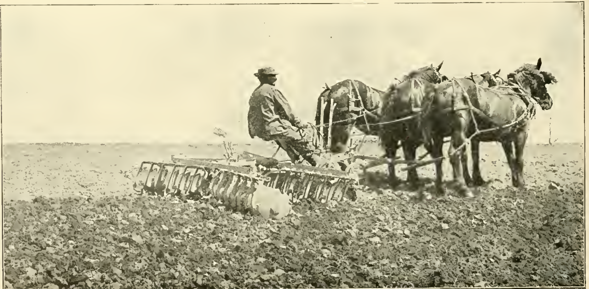
The McCormick disk harrow with the tandem attachment prepares a good seed bed in a short time
