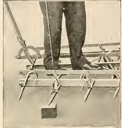
A harrow equipped with this strengthening bar will not bend even under the weight of a heavy man
