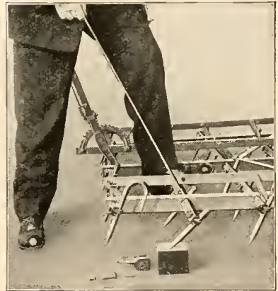
This is what happens to a harrow not equipped with strengthening bars when it strikes an obstruction
