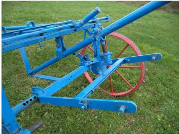
*Image 15: the tool carrier with removed toolbar.*
